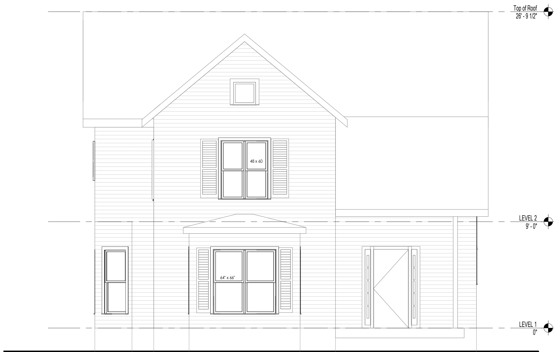
2 SOUTH ELEVATION A.20 SCALE: 1/4" = 1'-0"
