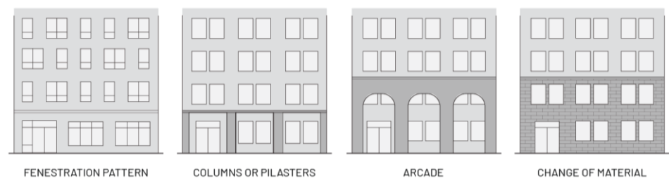
Figure 604-N. Building Base Articulation
