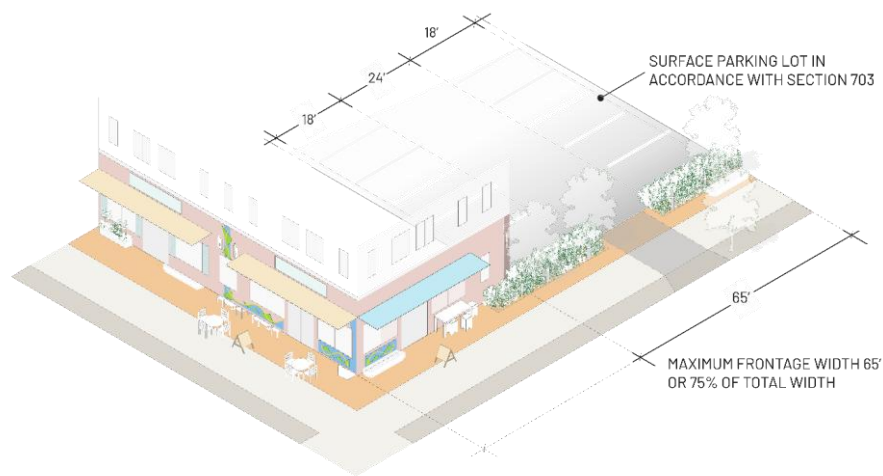
Figure 608-N. Surface Parking Frontage Maximum Width
