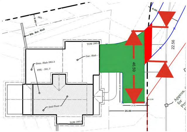
Figure 1: Section of site plan demonstrating proposed driveway dimensions. Area A (red) has a maximum width of twenty (20) feet, and Area B (green) has a maximum width of thirty-seven and a half (37.5) feet, both of which are exceeded by the proposed design.
