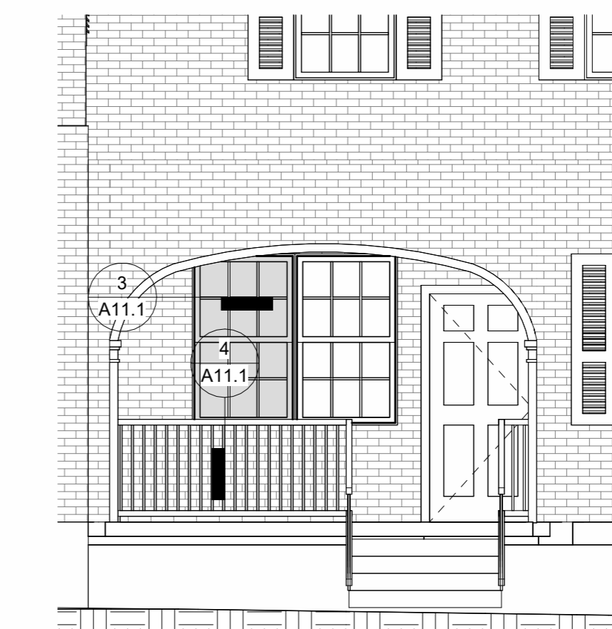
4 EAST ELEVATION VESTIBULE 1/4" = 1'-0"
