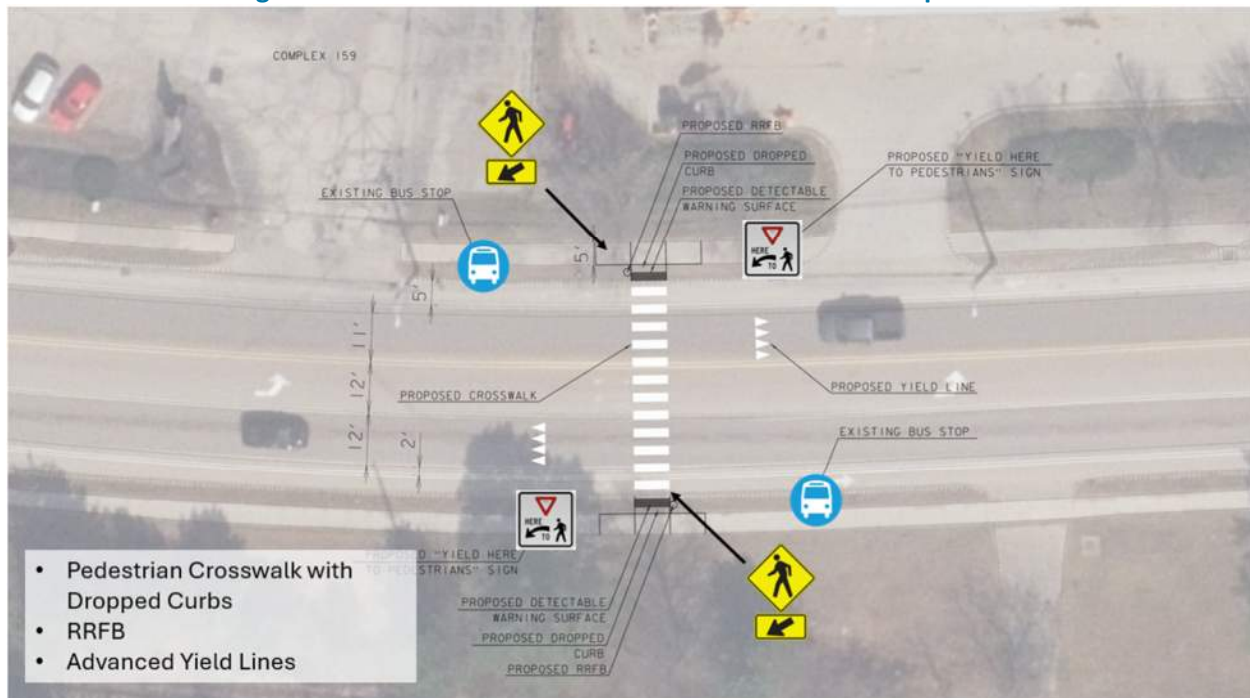
Figure 4 – Alternative 4 – Crosswalk with RRFB near Complex 159
