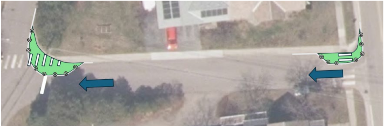
Figure 3: One-way traffic pattern originally proposed for this project. This pattern was ultimately not pursued as a part of the project design.
