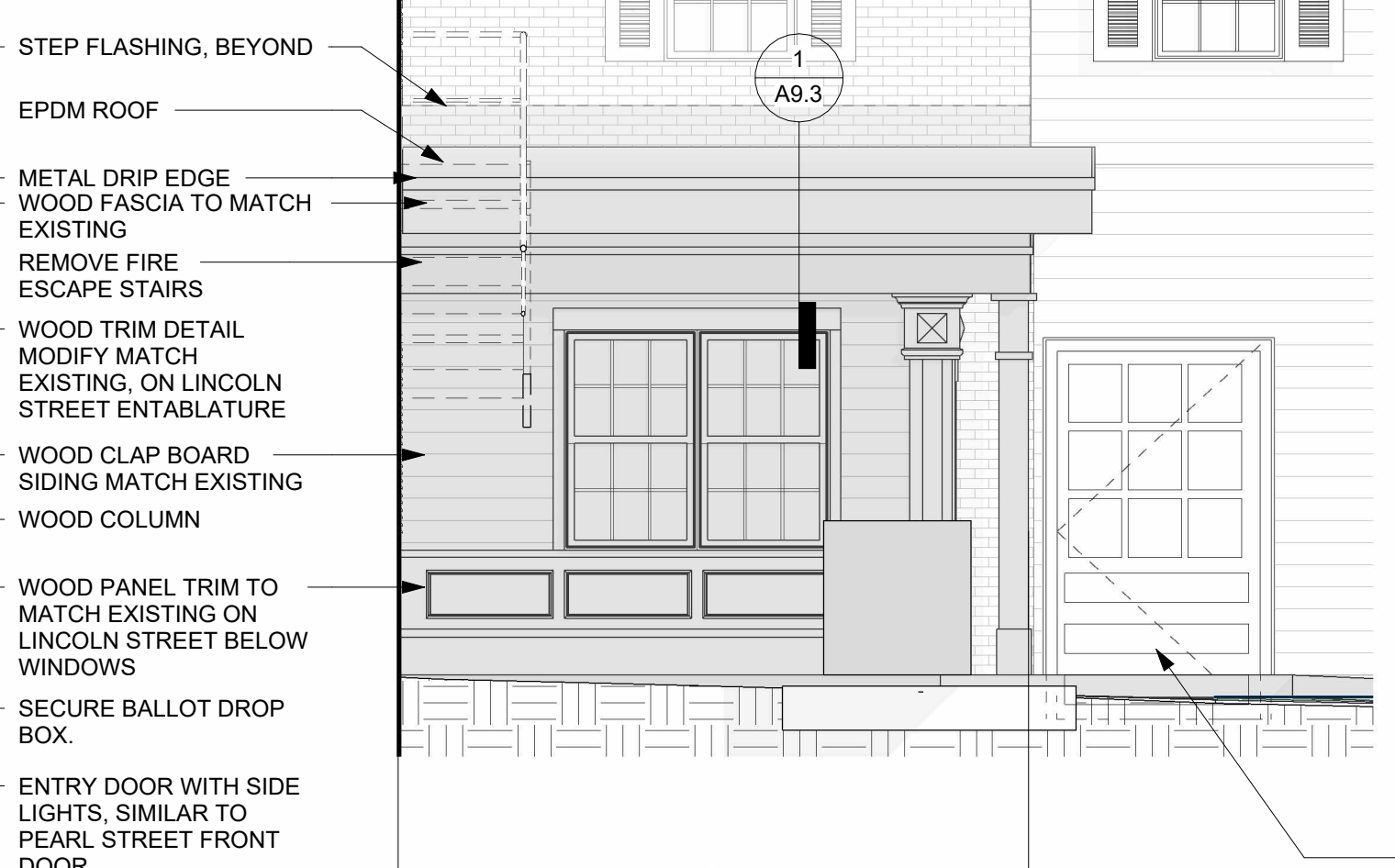
1 NORTH ELEVATION VESTIBULE 1/4" = 1'-0"
