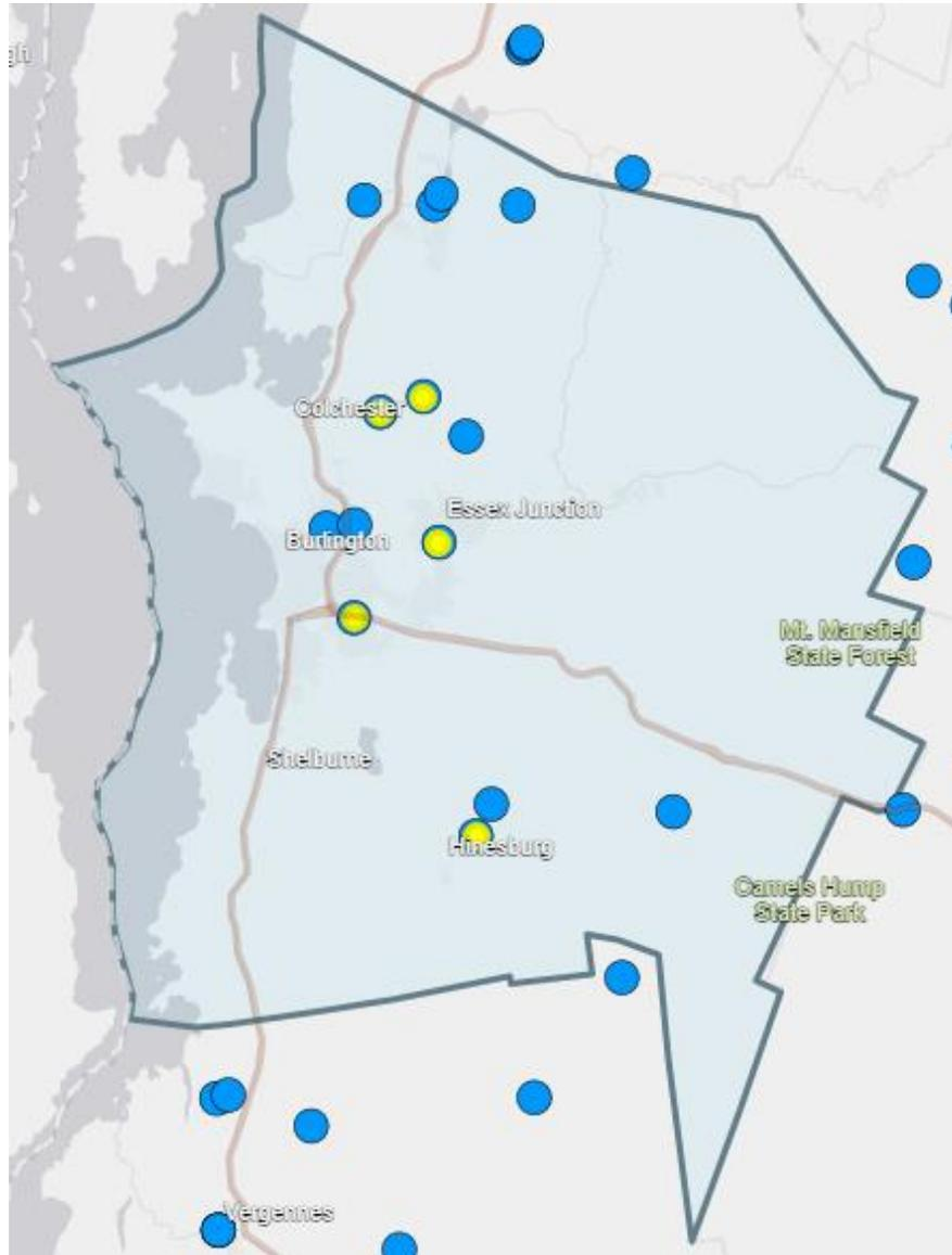
**Figure 4.1.3: National Inventory of Dams Significant Hazard Dam Locations in Chittenden County<sup>48</sup>**
