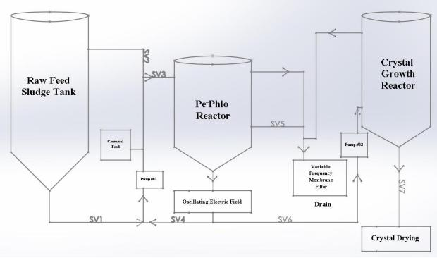
Figure 4. Phase II Updated Continuous Flow Pe<sup>-</sup>Phlo reactor design.
