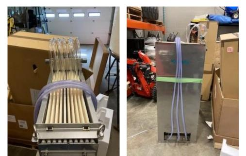
Figure 7. Pe<sup>-</sup>Phlo MBR (Membrane BioReactor) membrane to be retrofit with the oscillating AC field.
