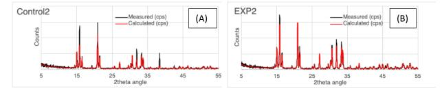
**Figure 6**. XRD spectra of struvite crystals in Control (A) and HydroFLOW-treated samples (B). XRD analysis confirmed that struvite crystals were of much more crystalline and better quality than the control samples.
