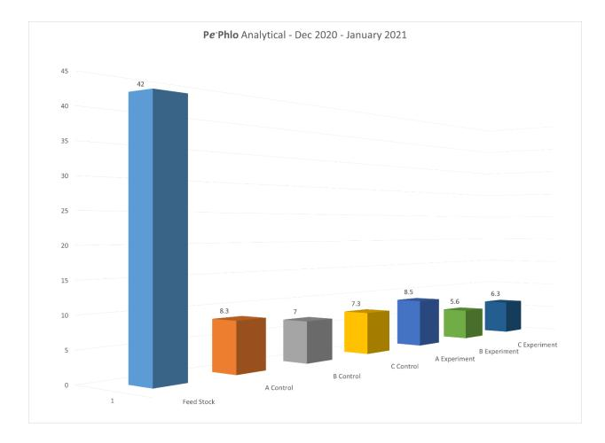
**pH Profiles** during three separate runs, A, B, and C (Experiment: HydroFLOW and Control (no HydroFLOW).
