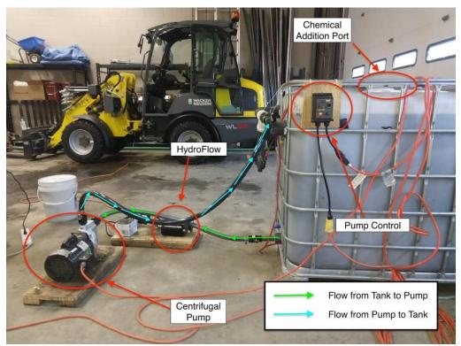
Figure 2. IBC pilot. UVM Capstone **Pe<sup>-</sup>Phlo** project. The student team used this reactor tank optimize process parameters including water chemistry and hydraulic characteristics.
