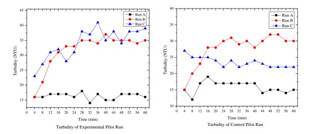
**Turbidity Profiles** during three separate runs, A, B, and C (Experiment: HydroFLOW and Control (no HydroFLOW).
