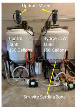
Figure 3. Phase II Updated short cycle Batch Pe<sup>-</sup>Phlo Reactor assembly with updraft mixers
