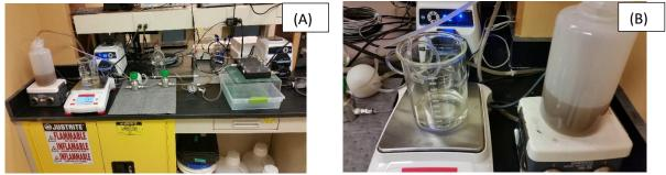
Figure 1. Laboratory scale  $Pe^-Phlo$  device (A). Products of  $Pe^-Phlo$  treatment include recovered reusable water (in the beaker) with the feed stock in the plastic bottle (B).
