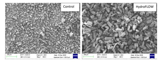
**Figure 5**. FESEM images struvite crystals in Control and HydroFLOW-treated samples. In HydroFLOW-treated samples the crystals are five-fold larger in size, better quality, and greater amount than the Control samples.
